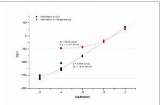
Pic. 3: Different calibration behavior for Magnesium sensor in different solutions with different ion background. The effect on different free fractions of Magnesium
