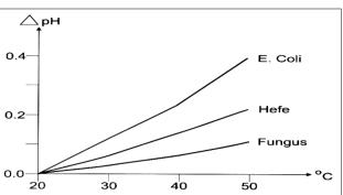
Pic. 4: Different behavior of pH values according the temperatur in different cell cultures. This matrix effect of pH / Temperatur dependencies can not be adusted by temperatur control.
